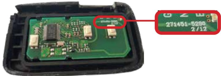
The next determining factor in selection is the remote frequency. Use your Key Tool Max to check the frequency and choose the XHORSE pathway that matches the Number & Frequency.
